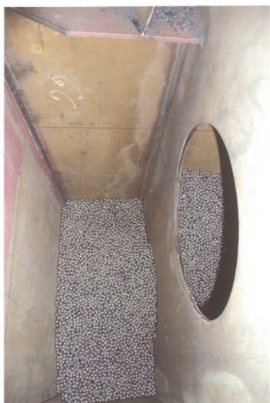
Lead shot ballast in stern
